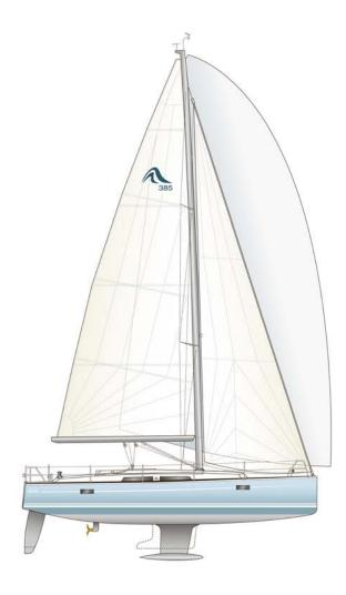
LOA 11.40 m | 37'4" Hull length 10.90 m | 36'06" LWL 10.40 m | 34'12" Beam 3.88 m | 12′73″
