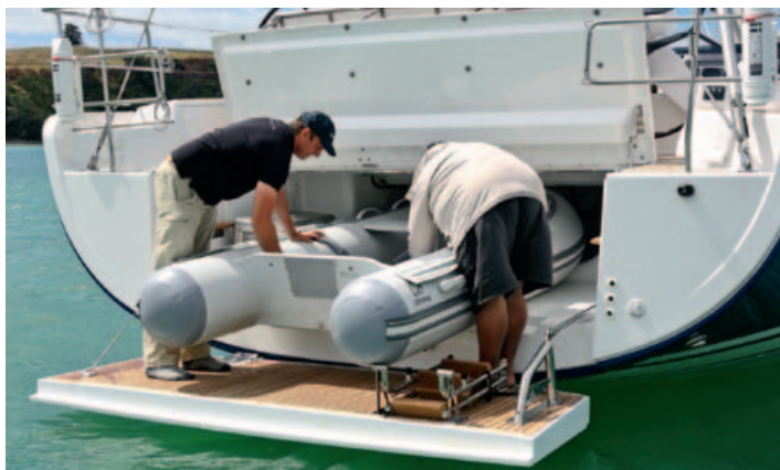
A 3m Zodiac fits into the transom garage; launching and retrieving is aided by the large, fold-down swim platform.
